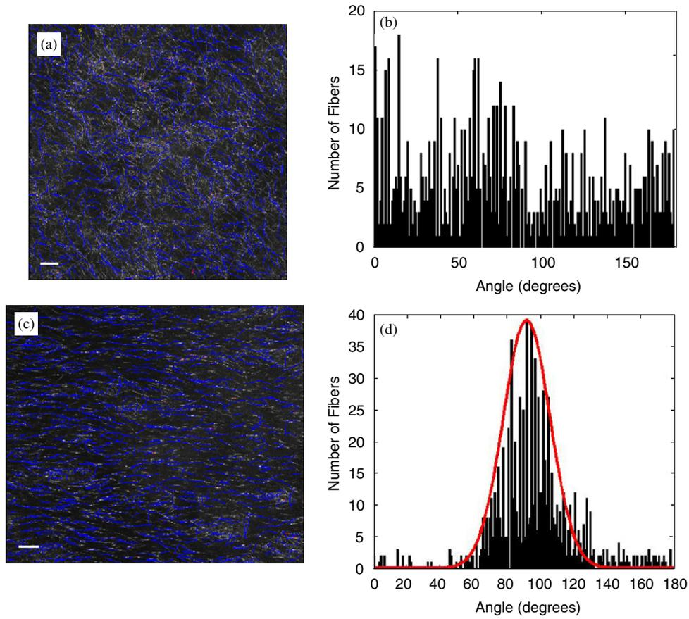
Fig. 2. [Color online.] (a) Fig. 1b overlaid with fibers identified by a program written for this purpose (blue). (b) Histogram of the angular distribution of fibers in Fig. 2a. (c) Image of aligned collagen fibers shown in Fig. 1c overlaid with identified fibers (blue). (d) Histogram of the angular distribution of fibers in Fig. 2b. Scale bar is  $15\mu\text{m}$  in both images.
