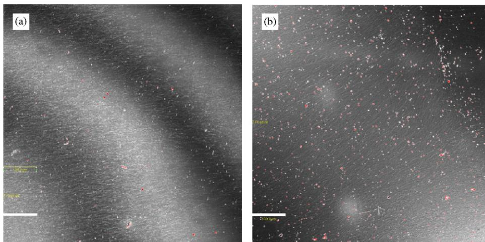
Fig. 3. (a) Low-magnification CRM image of a well-aligned thin gel. Striations are due to Airy rings as well as constructive and destructive interference from reflections from glass above and below the thin gel. (b) Low-magnification DIC image of a well-aligned thin gel. Both images are collected with a  $20\times$  objective. Scale bar is  $100\mu\text{m}$  in both images.
